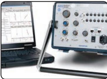
The **ultrasonic IRIS** option is used to inspect a wide range of materials including ferrous, nonferrous, and nonmetallic tubing. This technique detects and sizes wall loss resulting from corrosion, erosion, wear, pitting, cracking, and baffle cuts.
